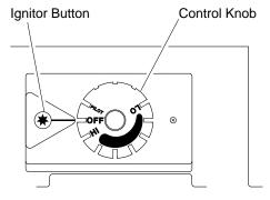
Figure 28 - Control Knob In The OFF Position
